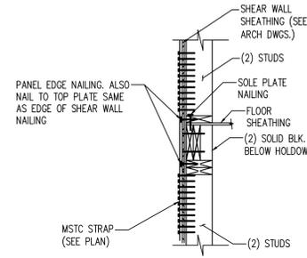
3 SHEAR WALL DETAIL W/ SIMPSON MSTC STRAP HOLDOWN (PER PLAN)
