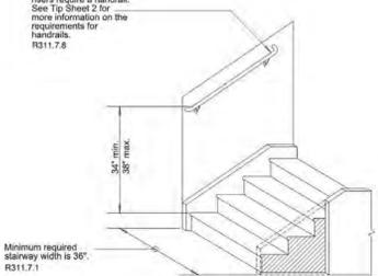
Figure 2: Typical Stair Elevation
