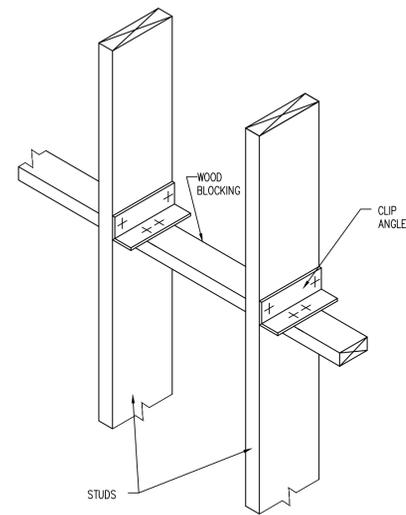
5 TYPICAL BRIDGING AND BRACING - CONTINUOUS BRIDGING
