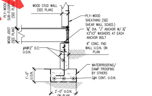
10 TYPICAL NEW CONCRETE FOUNDATION WALL SECTION
