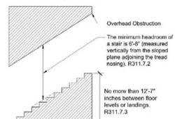
Figure 3: Headroom Clearance Requirements
