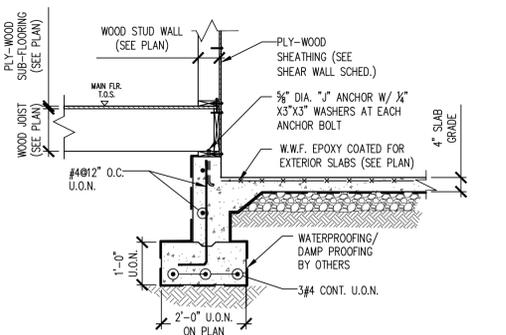
12 TYPICAL NEW CONCRETE FOUNDATION WALL SECTION
