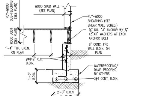
11 TYPICAL NEW CONCRETE FOUNDATION WALL SECTION
